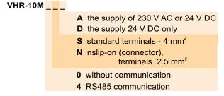
The VHR-10MxxD unit can be supplied by SELV voltage of 19-28 V DC; 60 mA. In addition to 19-28 V DC, the VHR-10MxxA unit can also be supplied with the voltage of 200-250 V AC; 50 mA. Simultaneous connection of both types of supply is impossible. When using the supply from 230 V AC, the output voltage of 20-24 V DC can be used for supplying probes. The direct current of 24 V DC can be replaced by a back-up battery which must have its own SELV charging source dimensioned according to its capacity.
