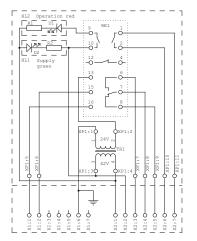
Example of the SOD-01 control cabinet connection
